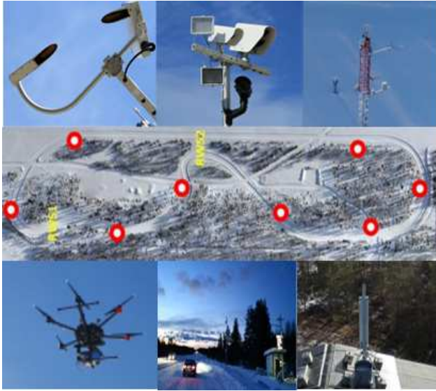
Fig.2 Test track equipped with 5GTN and ITS-G5, DAVN and IoT sensors with red spots
