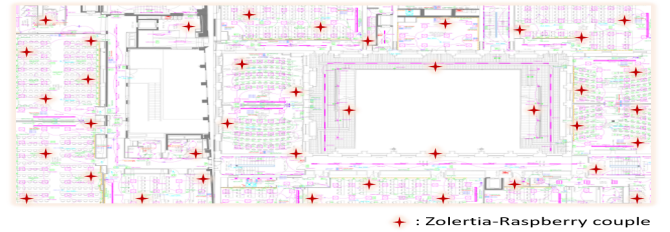
Fig. 1: Example of sensor deployment in one floor in the university
