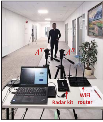
Fig. 2. Measurement setup for collecting RF sensing data and the trajectories of body segments during human walking experiment.
