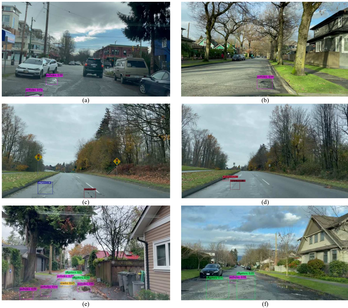
Fig. 3. Examples of road deterioration detection using (a), (b) YOLOX (c), (d) Swin Transformer and (e), (f) YOLOv4
