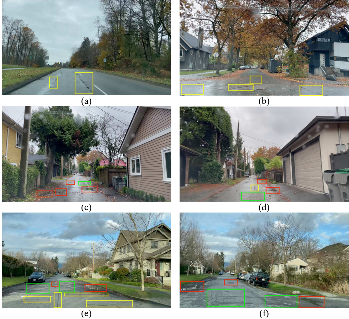
Fig. 1. Examples of labeled frames of our dataset, showing potholes in red, cracks in yellow and alligators in green.
