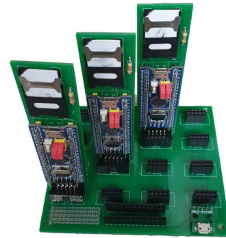
Fig. 8. A secure element grid, with 4x4 SEP slots. The estimated bus capacitance is 250 pF (450ns rise time for 1,8 k \Omega I 2 C Rp resistor)
