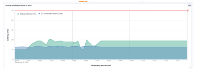
Fig. 5. Latency predictions vs actual values during static test
